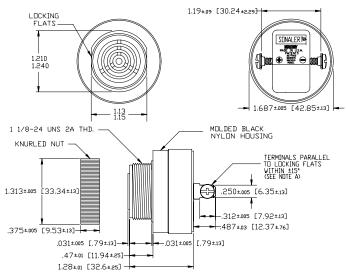
NOTE A: TERMINALS-032 BRASS TIN PLATED, TAPPED FOR #6-32 SCREW, TWD #6-32 NICKEL PLATED BRASS SCREWS INCLUBED, WILL ACCEPT 1/4\* QUICK CONNECT. NOTE B: MOUNTING- REMOVE BLACK PLASTIC NUT AND INSERT THREADED FRONT THROUGH 1.25' HOLE PUNCHED IN PANEL, IF DRIENTATION IS NEDED, NOTE LOCKING FLATS ON DRAWING. SCREW NUT BACK ON. DO NOT OVERTIGHTEN.
